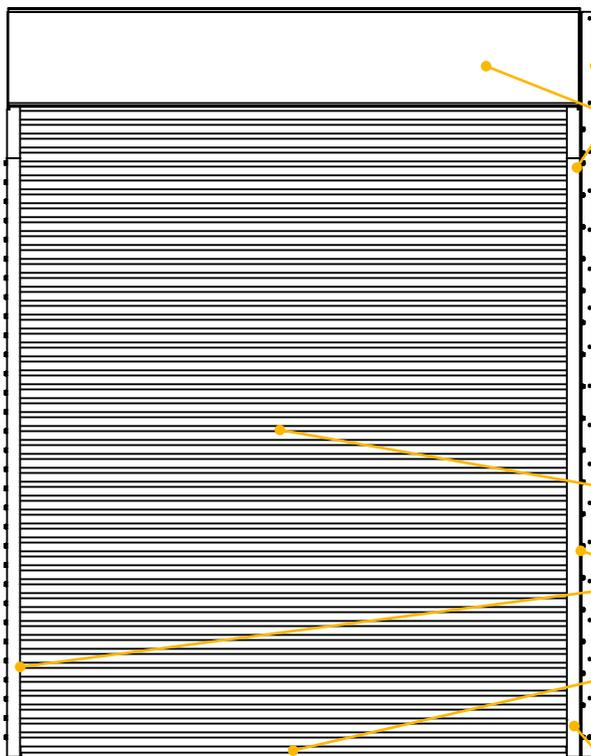
**PATENT PENDING WINDLOCKS** - Cut into the ends of each slat to engage in the windlock bar. Prevents the curtain from pulling out of the guides during high pressure events.
